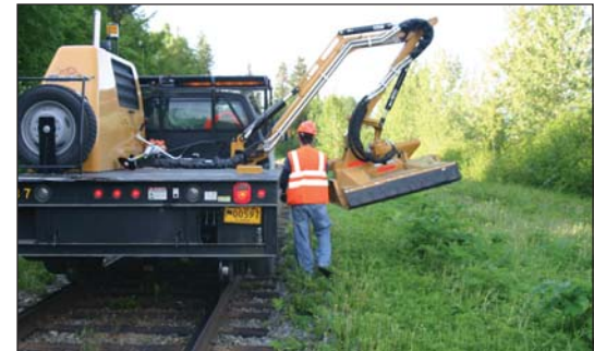
A rail-mounted brush cutter provides one method of mechanical vegetation control.
