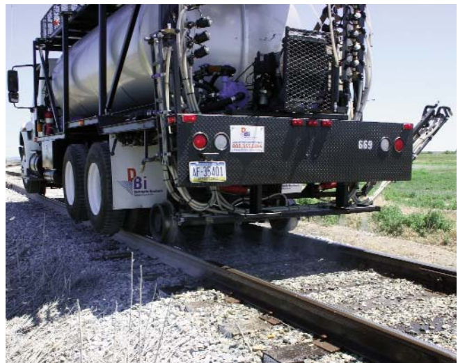
The DBI Company is an industry leader in railroad vegetation management nationwide. DBI's specially-equipped trucks direct weed control products directly at the track bed.
