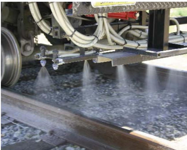
The DBI Company is an industry leader in railroad vegetation management nationwide. DBI's specially-equipped trucks direct weed control products directly at the track bed.
