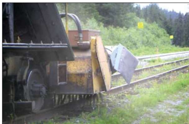
Above and right: The ballast regulator's bristles are normally covered with rubber. The rubber is stripped to expose the wire when the ballast regulator is used for vegetation management.
