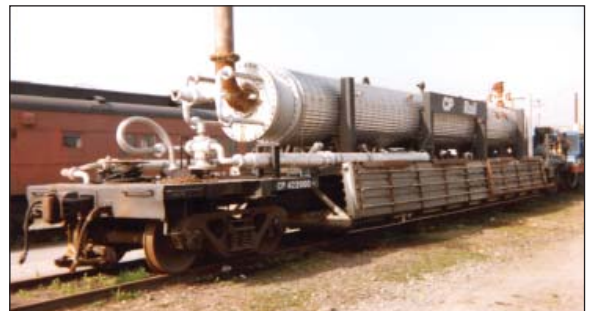
The CP Steam Machine steam / boiler car.
