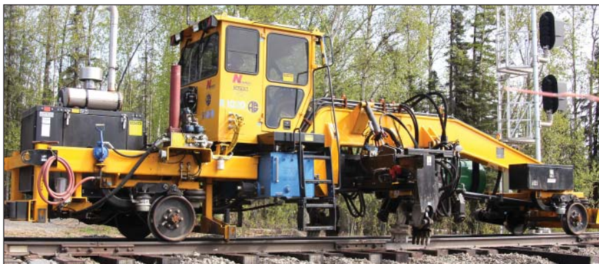
A tie remover/inserter has powerful mechanized arms (close-up, right) that can extract old, and install new, ties from either side.
