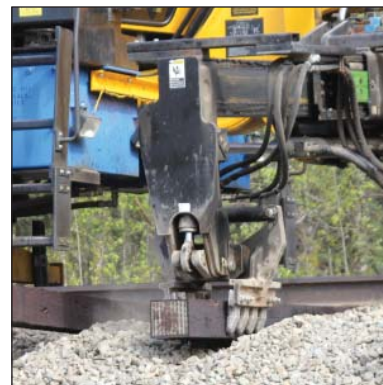
A tie remover/inserter has powerful mechanized arms (close-up, right) that can extract old, and install new, ties from either side.
