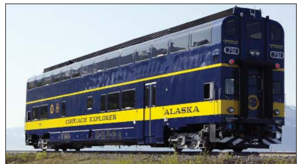
The self-contained, self-propelled DMU.
