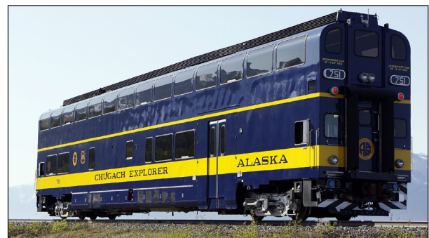
The self-contained, self-propelled DMU.
