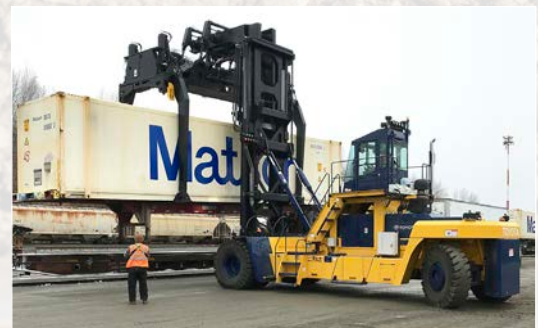
A brand new van loader is put to work, supporting the Anchorage Trailer on Flat Car (TOFC) business.
