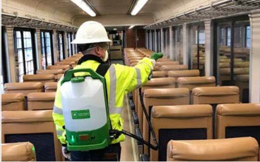
Janitorial contractor ESS uses a stabilized aqueous ozone (SAO) mist to sanitize passenger train interiors.
