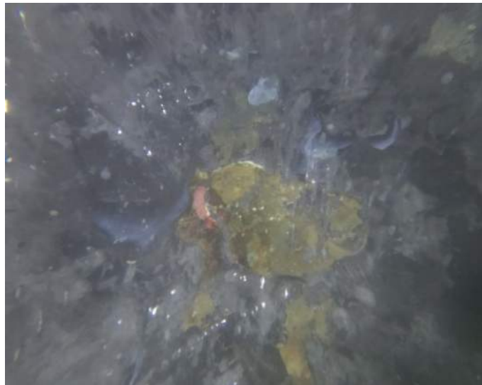
Image 15 - Close up of pitting and corrosion
