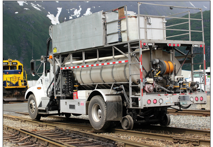
The contractor applies herbicides using a rail-equipped vehicle outfitted with low-volume, low pressure nozzles and attachments to apply herbicides with precision.
