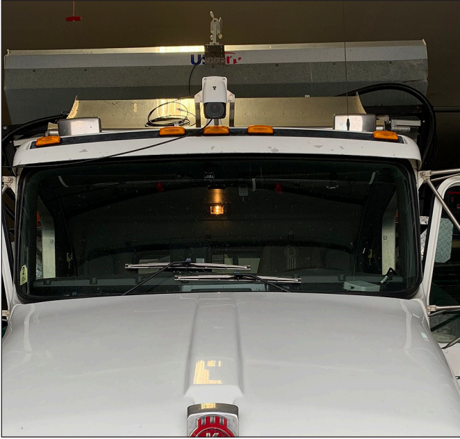
The Ricospray infrared camera is mounted on top of a truck cab, to provide a clear vantage point for detecting weeds.
