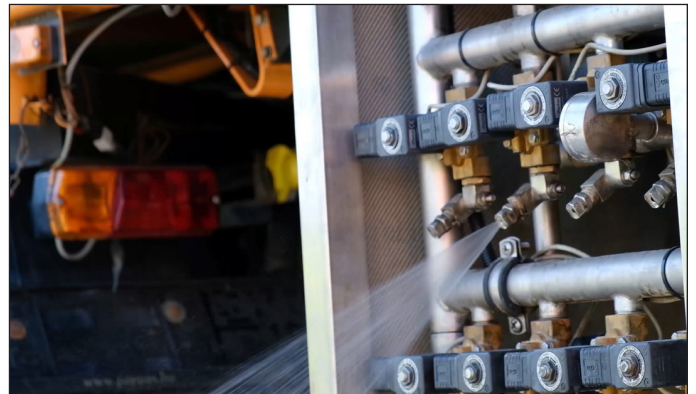
The contractor applies herbicides using a rail-equipped vehicle outfitted with low-volume, low pressure nozzles and attachments to apply herbicides with precision.
