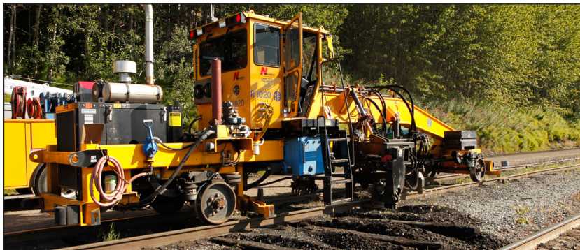
A tie remover/insertor has powerful mechanized arms (close-up, right) that can extract old, and install new, ties from either side.
