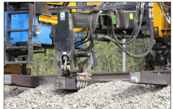
A tie remover/insertor has powerful mechanized arms (close-up, right) that can extract old, and install new, ties from either side.
