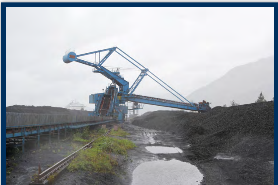
Photo IV-3.3: SLF Stacker/Reclaimer and Conveyer (Source: Judy Patrick Photography, 2012)
