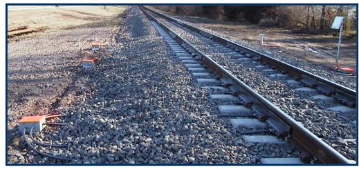
The WILD device strain gauge and cables are installed along the rail, with cable conduit leading to trackside junction boxes and system electronics.
