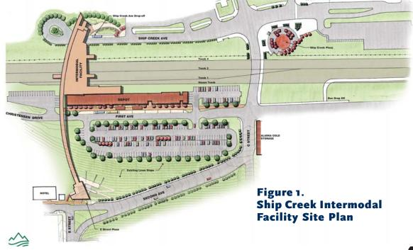
Since constructing a parking garage is not feasible, upgrades to the existing parking lot have been designed. To meet current municipal standards for parking lots, including size of parking stalls and adequate circulation and access, and to provide landscaping to enhance the appearance and provide a buffer between the parking lot and the park, a small area of the Quyana Park (approximately 0.25 acres) would be used.
