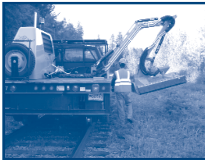
L-R: One of two new brush-cutters mows weeds to about 6 inches high on a stretch between Girdwood and Portage. Five weeks later, most weeds had grown to nearly two feet tall and some grew several feet. Such growth requires multiple brush-cutting throughout the summer.
