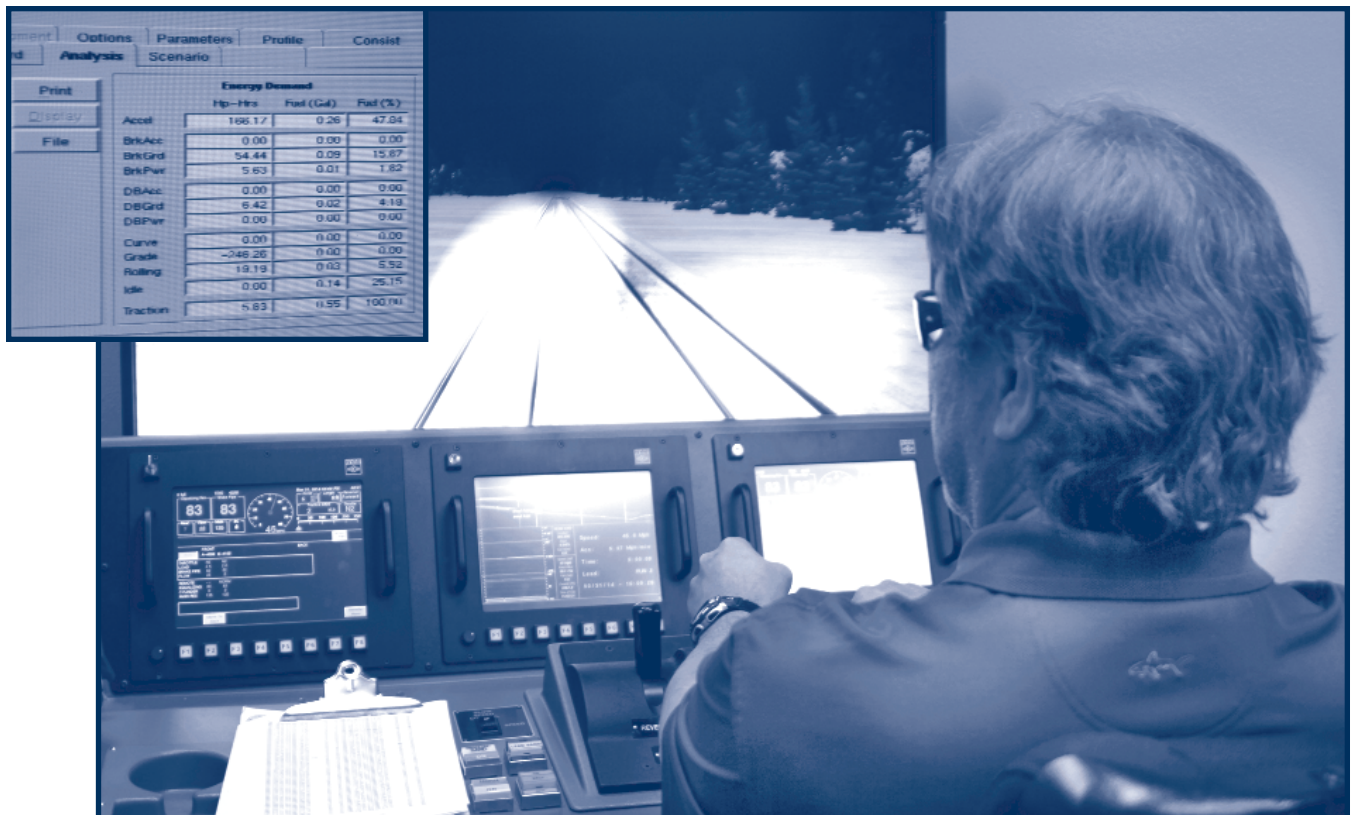
Veteran Train Engineer Frank Shepard demonstrates how to operate the SD70MAC locomotive simulator. Inset: Located behind the simulator operator’s seat, the Engineer Supervisor sits with access to a monitor that shows simulated locomotive energy demand factors, such as acceleration, horsepower, fuel used and fuel efficiency.
