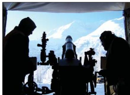
**A Howitzer gun is used to trigger a controlled slide.**
