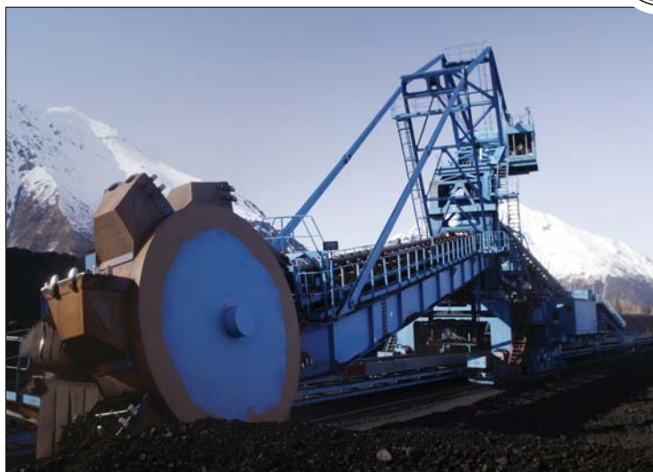
The reclaimer collects coal from the stockpile to put on the conveyor.
