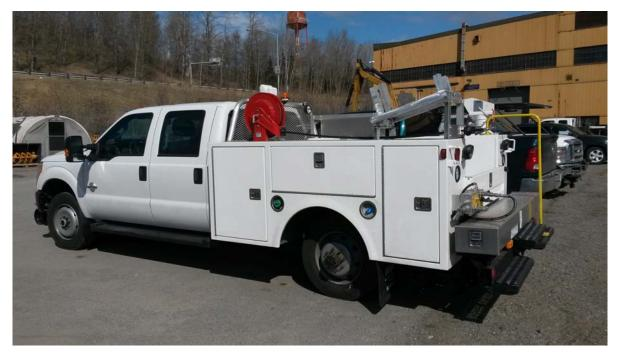
Headache rack with installation & wiring for spot light (1), beacon light (1) & external speaker
