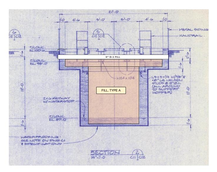
Figure 5: D-1 Aggregate over Fill
