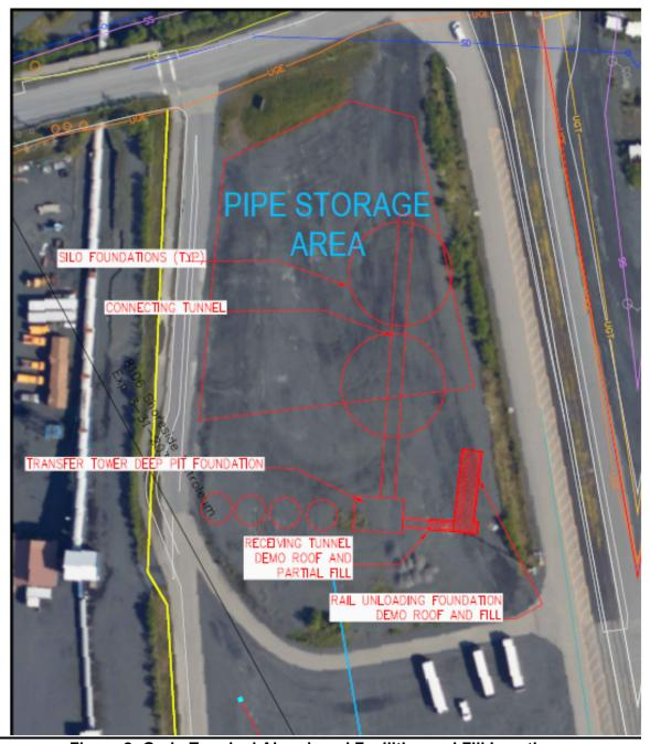
Figure 2- Grain Terminal Abandoned Facilities and Fill Locations
