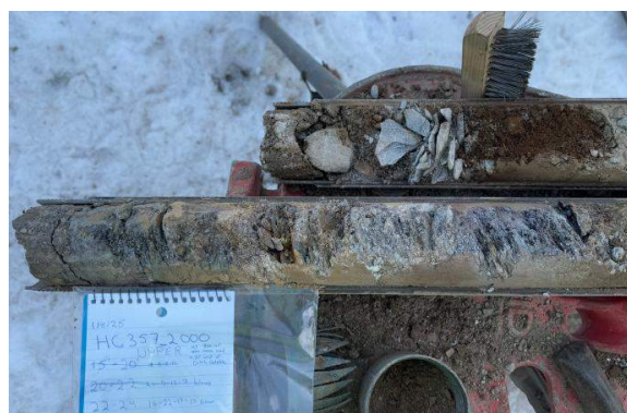
Photo 3.4: Borehole 20+00 ~25-ft East of ditch CL bedrock showing both samples recovered from 20 to 22-ft and 22 to 24-ft.
