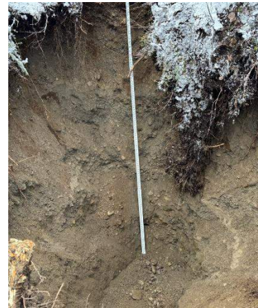
Photo 2.2: TP1D, STA 20+00 ~50 East of CL looking uphill. Bedrock not located in ~18-ft deep pit
