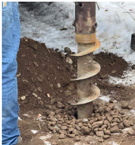
Photo 3.2: Boring the 18+50 borehole, surfacing tailings changed to small gravels at ~15 to 20-ft depth
