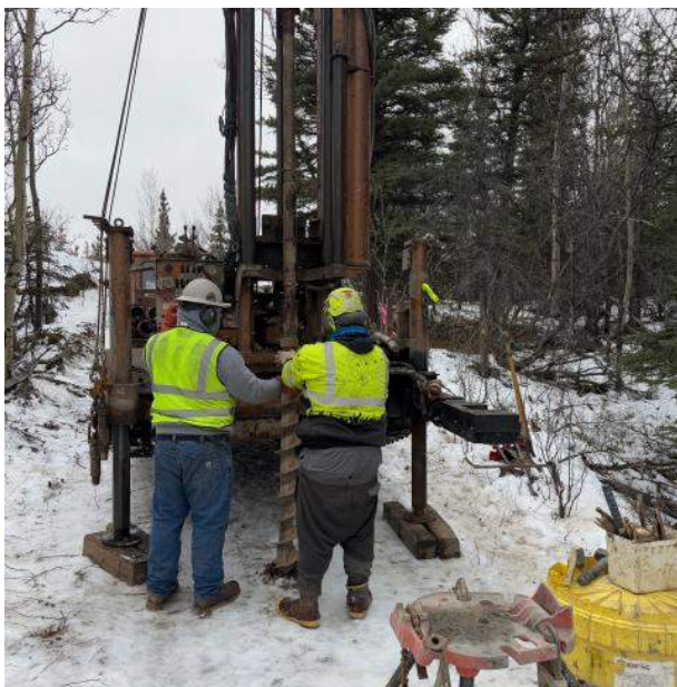
Photo 3.1: CME-850X Setup and operators drilling the 18+50 borehole
