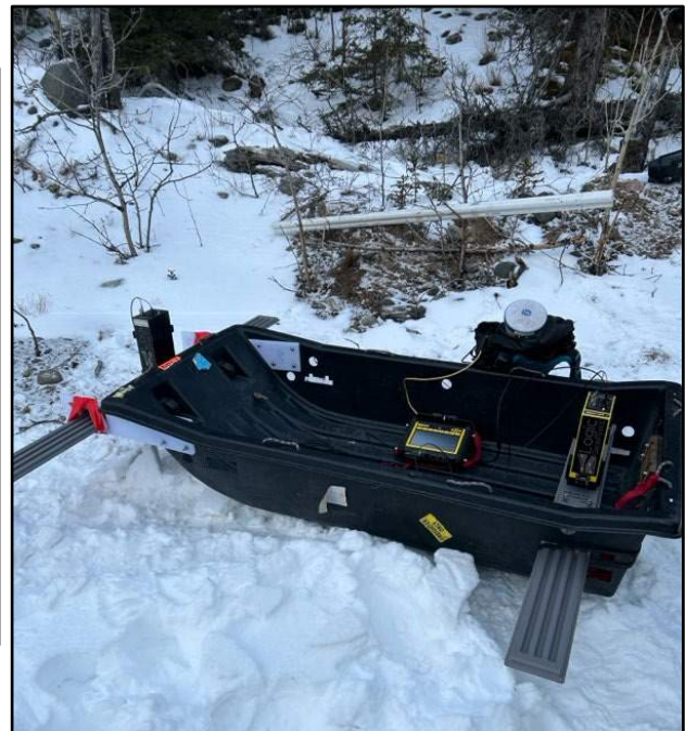
Photo 3: The 50-MHz GPR system on site in the perpendicular configuration.
