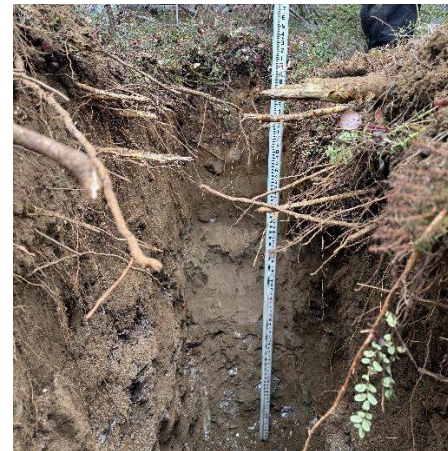
Photo 2.4: TP2, STA 18+00 above CL looking uphill. Bedrock located 5 to 6-ft below EG
