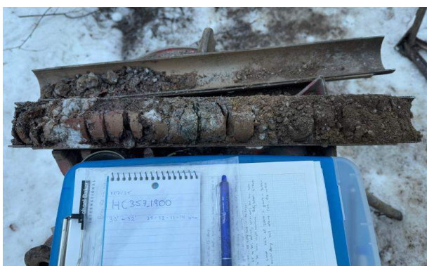
Photo 3.3: Borehole 19+00 bedrock sample recovered from 30 to 32-ft deep after rapid drilling to 30-ft depth. Transition from weathered bedrock to more intact rock fabric confirmed in subsequent 32 to 34-ft split spoon sample.
