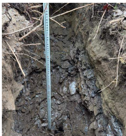
Photo 2.5: TP3, STA 15+50 on CL looking uphill, Bedrock located 5 to 7-ft below EG
