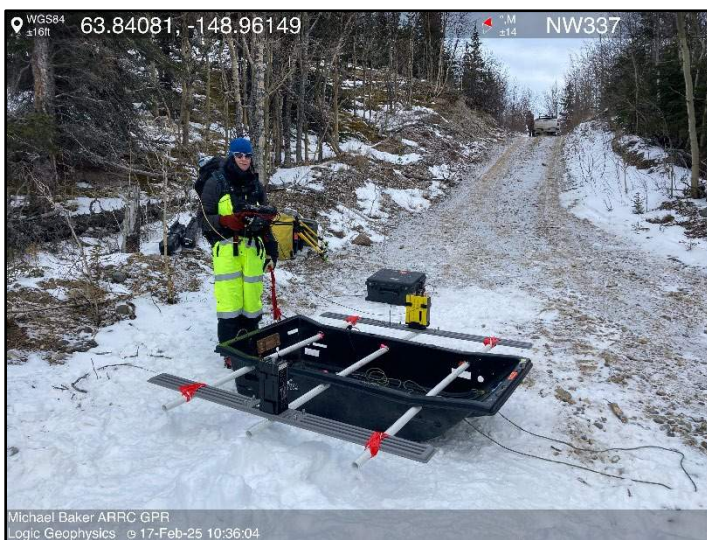
Photo 2: The 50-MHz GPR system on site in the parallel configuration
