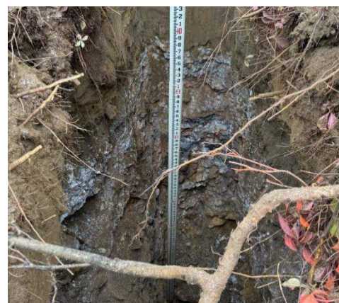
Photo 2.6: TP4, STA 13+50 above CL looking uphill. Bedrock located 2.5 to 3.5-ft below EG
