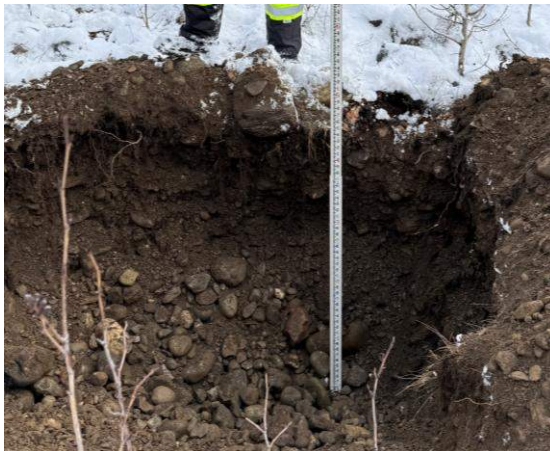
Photo 2.3: TP1U, STA 20+00 ~65' West of CL looking downhill. Bedrock not located in 5-ft pit
