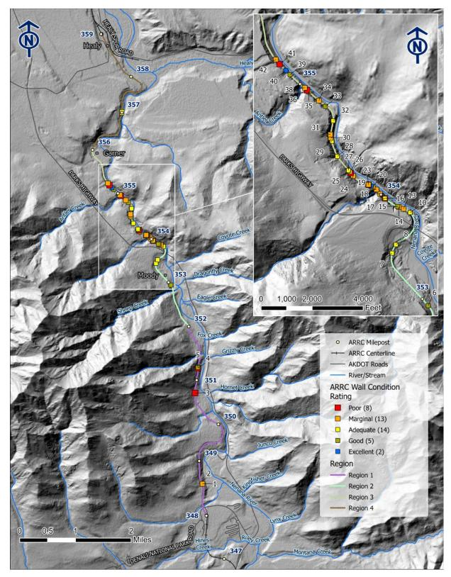
Figure 6-1: All Retaining Walls in Healy Canyon
