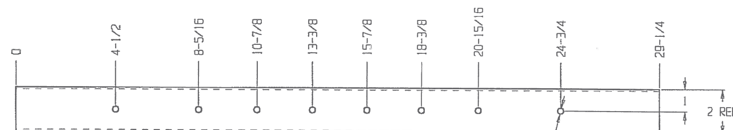
ITEM 6 FROM DWG: ARIA16IA1001 MATERIAL: 2" X 1" X 16GA A36 MILD STEEL TUBE
