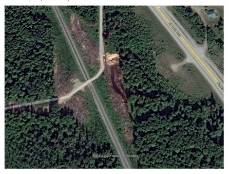
A: The cleared area is actually slightly larger than the sight triangles. ARRC Identify the general excavation area in a bid documents. There was "hump" of material within the sight triangle restricting line of sight down the tracks.
